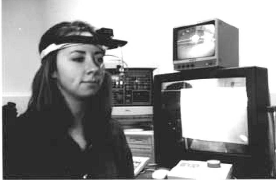
**Figure 2.** A subject wearing a light, head-mounted eye tracker. The eye monitor, with cross hairs on the pupil and corneal reflection is shown in the top right. The view from the scene camera, with the subject's point of gaze superimposed, can be seen in the bottom right.
